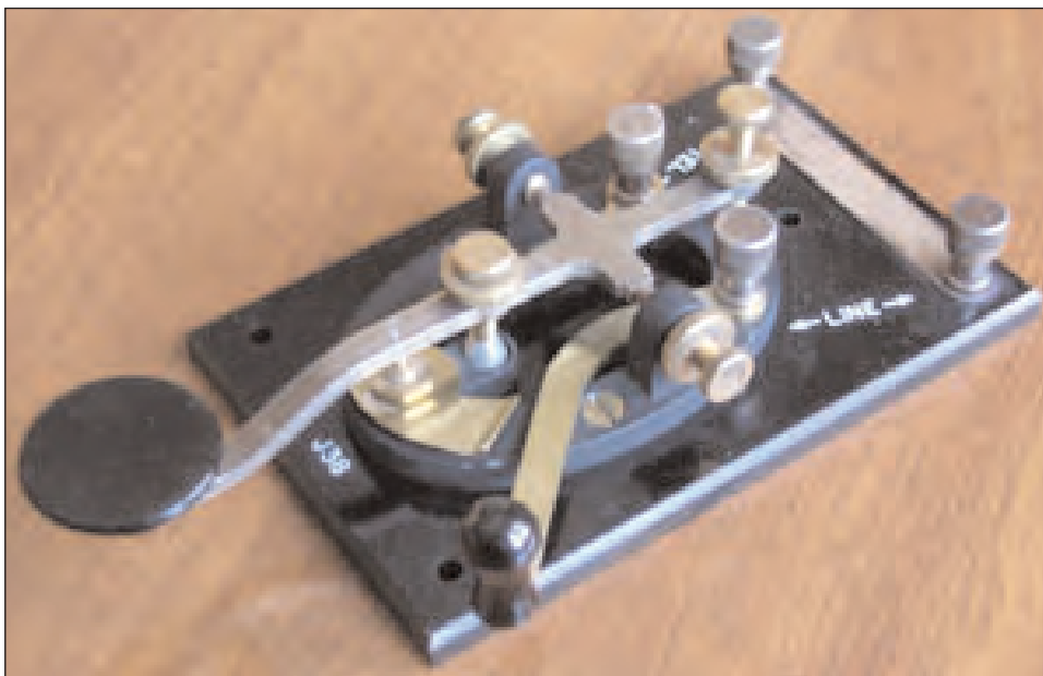
Sample Morse Code telegraph key. Used by permission of photographer Lou Sander
